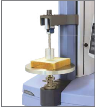
Compression Test on Bread
