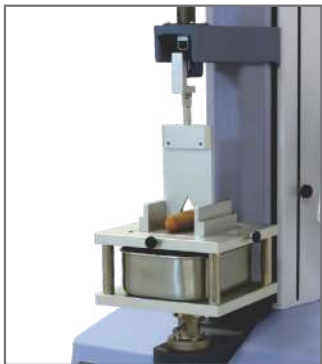
Shear Test on Sausage
